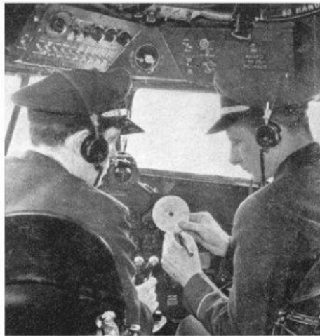
New type navigation computer in use during flight. With this instrument the pilot may quickly determine answers to flight problems arising during the course of the trip.
